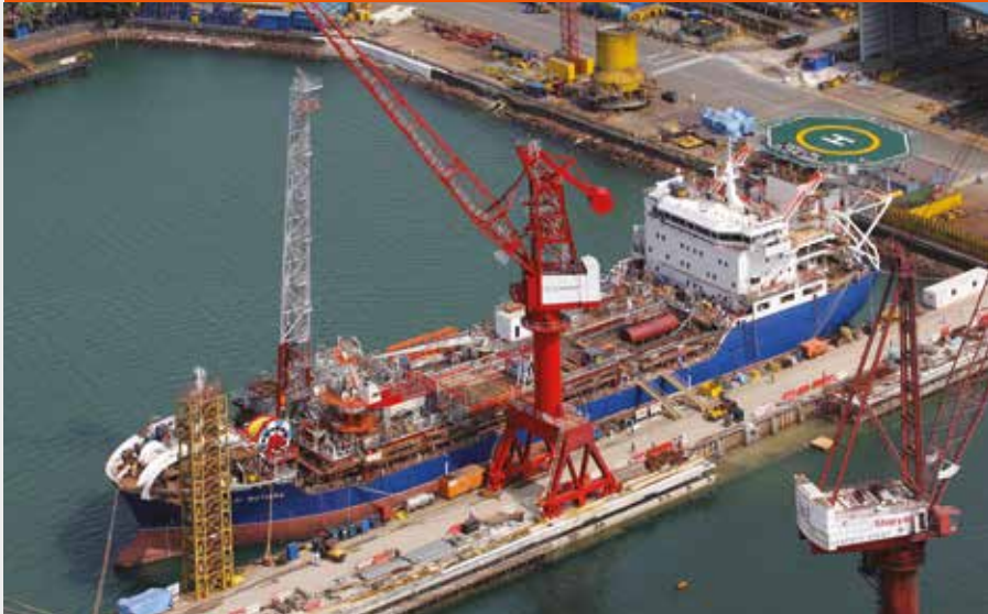
Conversion of Early Production Vessel
