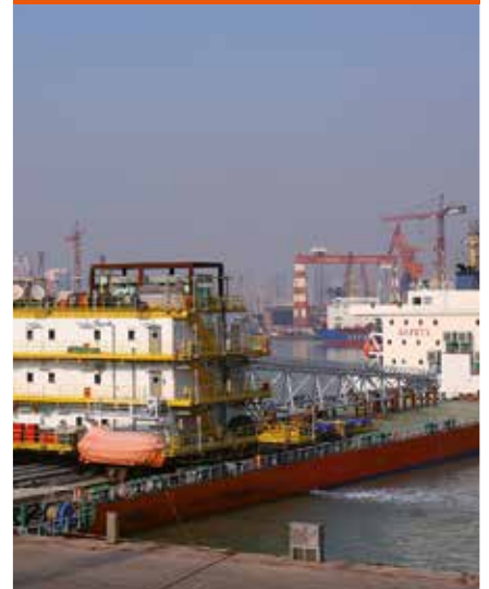
Platform living quarters loaded for transportation to location
