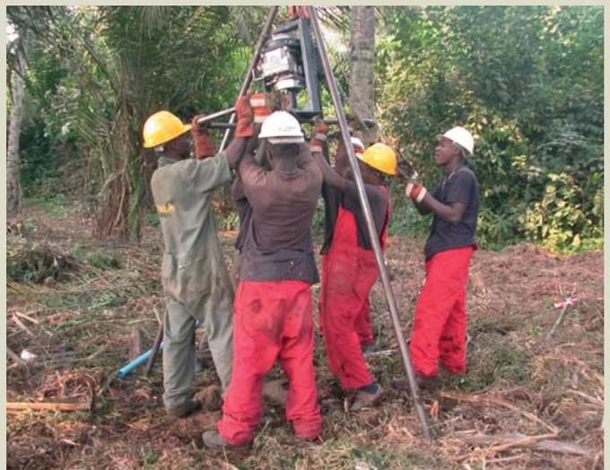
*Seismic crew drilling shot holes for the dynamite part of the 2005 seismic survey in the Cabinda South Block, onshore Angola.*
