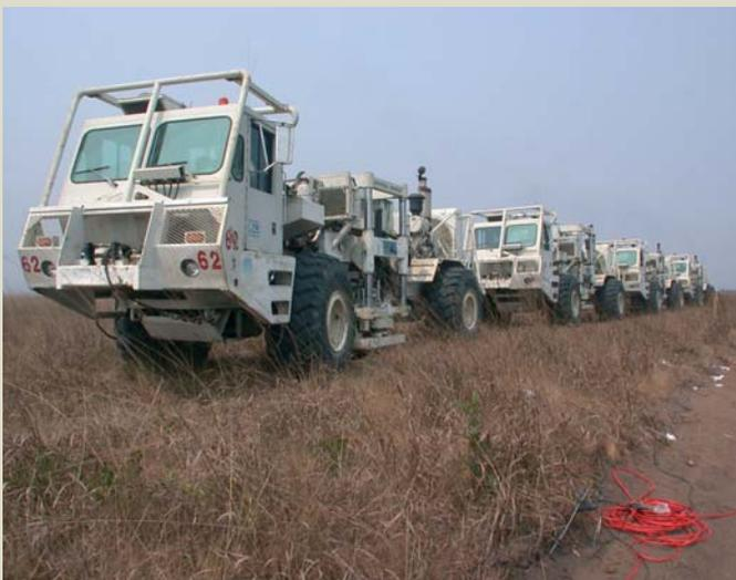
*Vibroseis trucks during the 2005 2D and 3D seismic survey in the Cabinda South Block, onshore Angola.*
