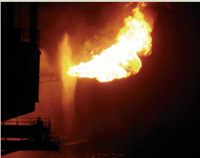
*This 2003 production test of Chinguetti-4-5 confirmed the field's commercial potential with a stabilised flow of up to 15,680 BOPD. It set the scene for the US\$750 million/A\$1,022 million Chinguetti Oil Field Development which produced first oil on 24 February 2006.*
