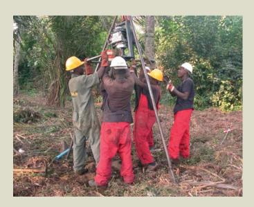
Seismic crew drilling shot holes for the dynamite part of the 2005 seismic survey in the Cabinda South Block, onshore Angola.
