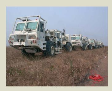
Vibroseis trucks during the 2005 2D and 3D seismic survey in the Cabinda South Block, onshore Angola.
